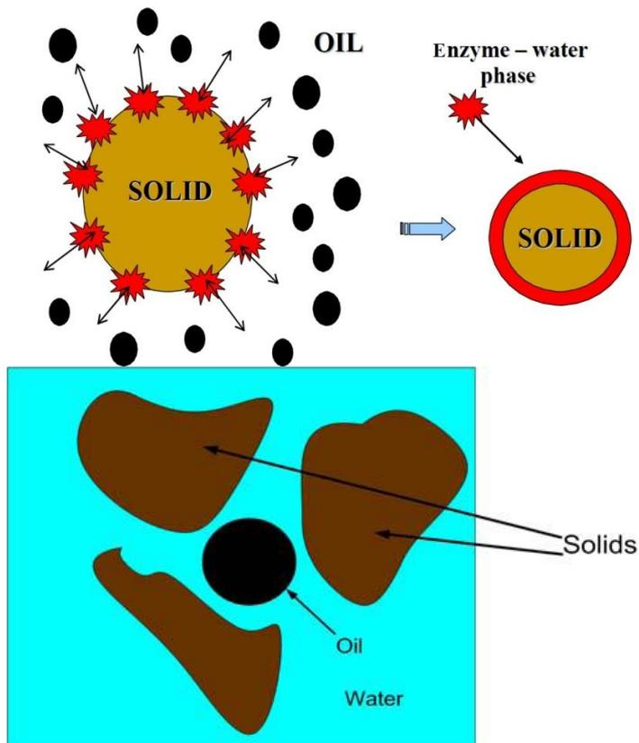
**Figure 4** – EEOR in water wet systems
