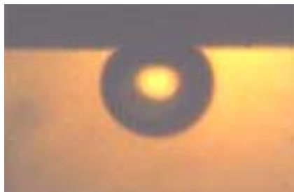
Limestone (initial): \theta = 133.64^\circ
