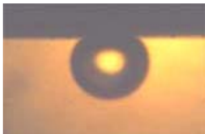
Limestone (5minutes): \theta = 132.49^\circ
