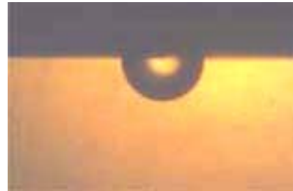
Sandstone (initial): \theta = 94.35^\circ
